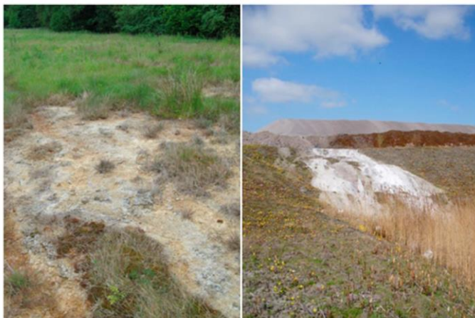
Figure 8. (left) A “hardpan” of carbonate formed on waste slag mounds at former steelworks in Consett, United Kingdom. (right) Carbonate precipitation in waters egressing from a waste landfill in Scunthorpe steelworks (photograph courtesy of Carla-Leanne
